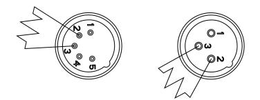
A DMX512 terminator reduces signal errors, avoiding most signal reflection interference. Connect PIN 2 (DMX-) and PIN 3 (DMX+) of the last fixture in series with a 120 Ohm, 1/4 W Resistor to terminate the DMX512.
